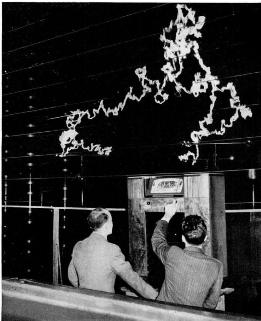
Figure 15: A 1940s demonstration of FM's robustness to noise. It reproduces a broadcast despite the 1 MV arc in the background. Source: Wikipedia.
